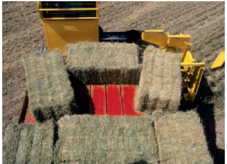
After you select or create a stack pattern that fits your needs, the bales are configured automatically.
