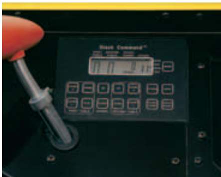
The Stack Command™ control system provides up to 35 pre-programmed stack patterns as well as room for 20 custom patterns that you can program.
