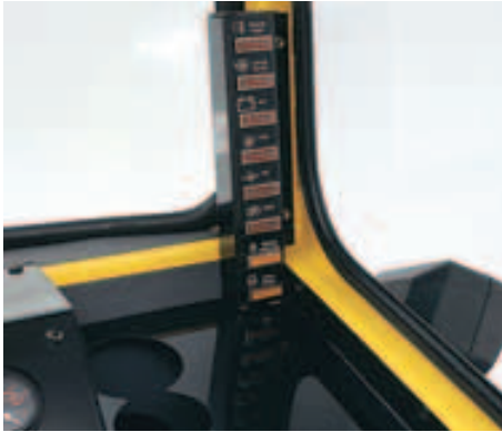
This warning light display tower provides information on key functions.
