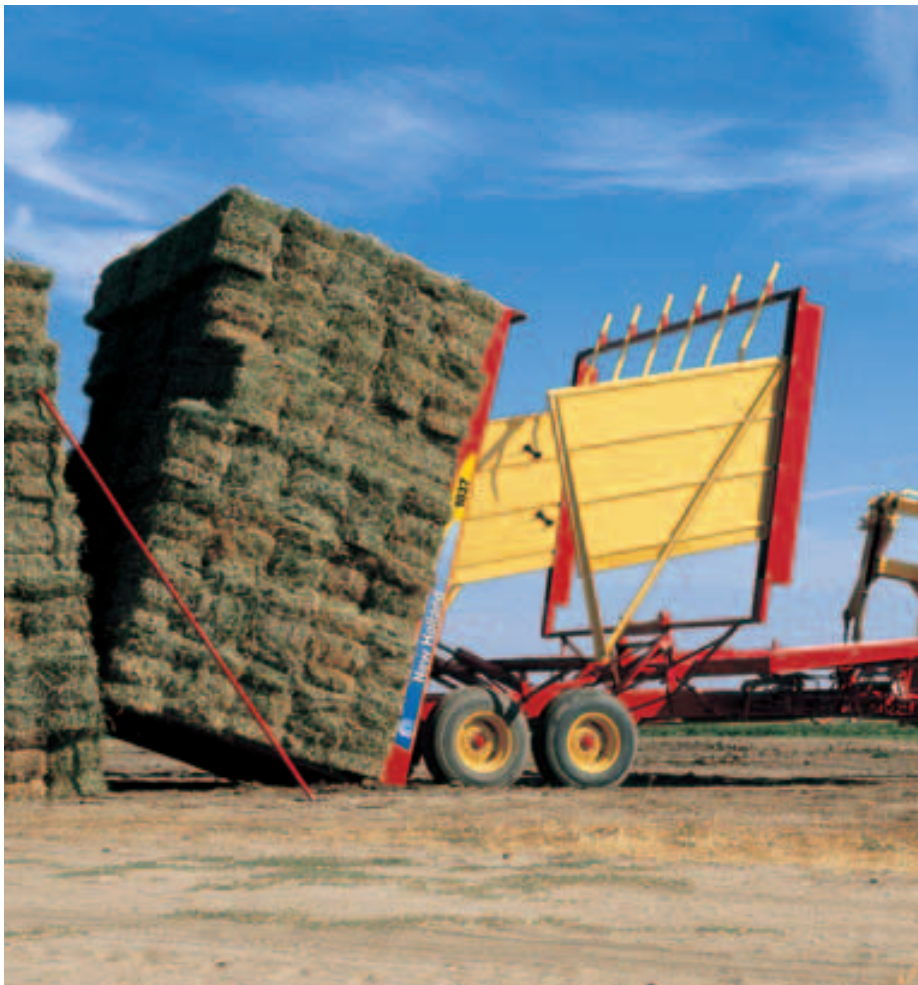
The Model 1037 handles about four tons per load – 104 14" x 18" bales or 83 16" x 18" bales.
