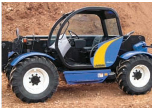
The LM5080 ROPS model features the same expansive visibility as the cab model. It is ideal for light construction use as a multi-purpose tool carrier.
