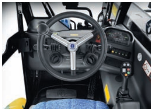
The roomy cab has grouped controls, a seat-mounted joystick, and standard high-capacity heating and air conditioning for maximum operator comfort.
